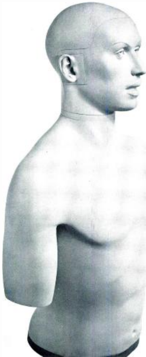
Figure 3. The complete KEMAR manikin provides life-like test conditions, primarily in research and development of hearing aid devices.
